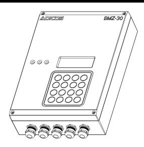
ADICOS BMZ-30 is one of three types of master units for the Advanced Discovery System ("ADICOS"), which was specifically designed to provide reliable early fire detection in industrial surroundings. It provides communication signals for up to 250 ADICOS detectors and builds the interface link between the ADICOS installation and the service-PC. This connection is based on RS-232 serial interface by default - ethernet and conventional modem extension modules are available.
