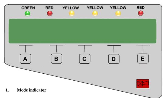
Green LED ON – normal operation. Green LED FLASHING – Control unit in test mode. Green LED OFF – power failure.
