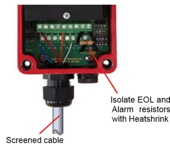
Figure 3. Control panel wiring
